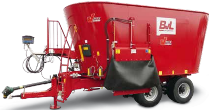
Two-auger mixer wagons with a large volume
